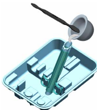
Figure 5. The cement delivery syringe placed at an angle to aid cement transfer from mixing bowl to syringe. The cement paste can run slowly down the barrel without trapping air inside the syringe and thereby create a more consistent end product.
